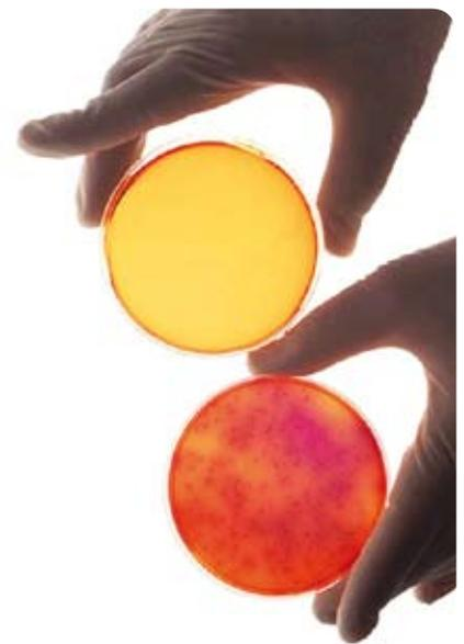
*Petri dish tests prove the destruction of harmful germs by **SilverProtec**<sup>®</sup> (upper petri dish germ-free)*
